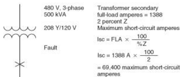
FIGURE 26.2.2.3.1 Example Calculation of Maximum Available Short-Circuit Current at the Transformer Secondary Terminals.
